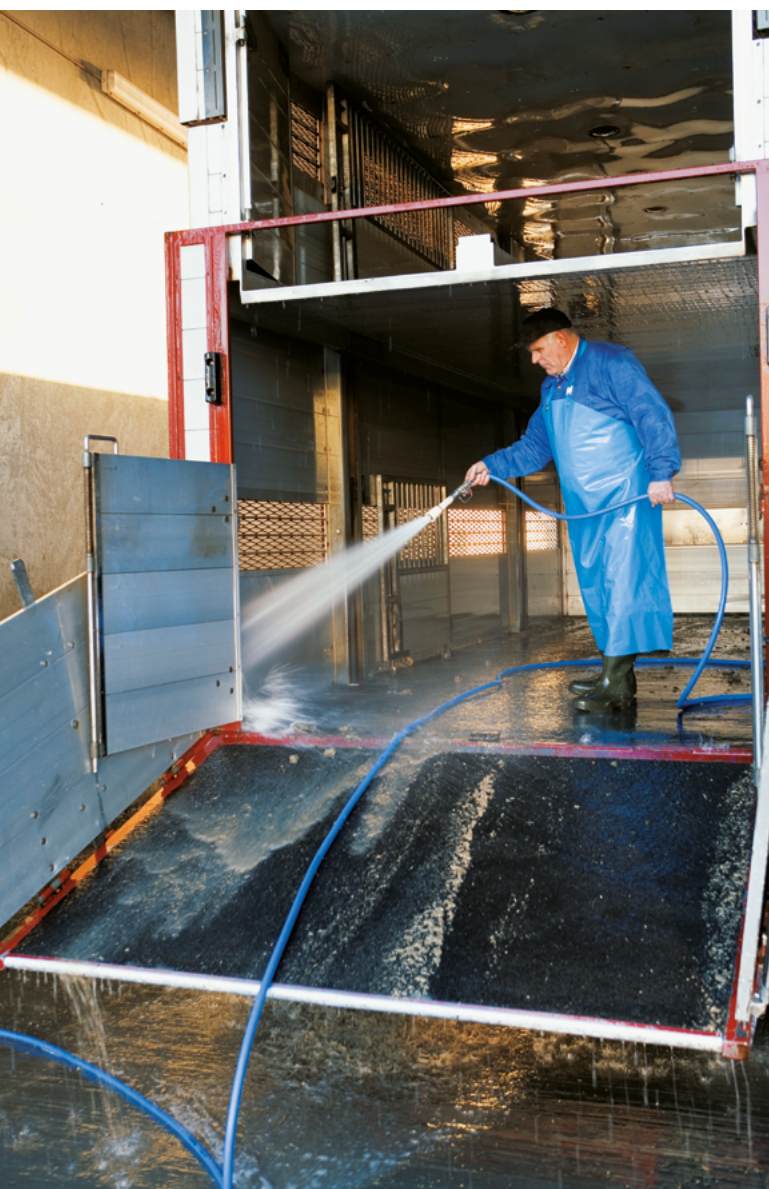
To minimize the risk of any disease spreading, all transport vehicles must be cleaned and disinfected after unloading and before leaving the slaughterhouse.
