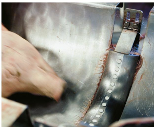
Autoform calculates the meat and fat content of the carcass, based on ultrasonic measurements. The measurements are performed by 16 transducers mounted on a channel over which the carcass passes once it has been transferred to the gambrel.
