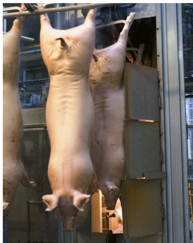
Typically, singeing of the carcass takes place in a furnace at 1000 °C for 6 seconds, thus eliminating bacteria, the remains of bristles and other dirt and preparing the surface of the rind for scraping.
