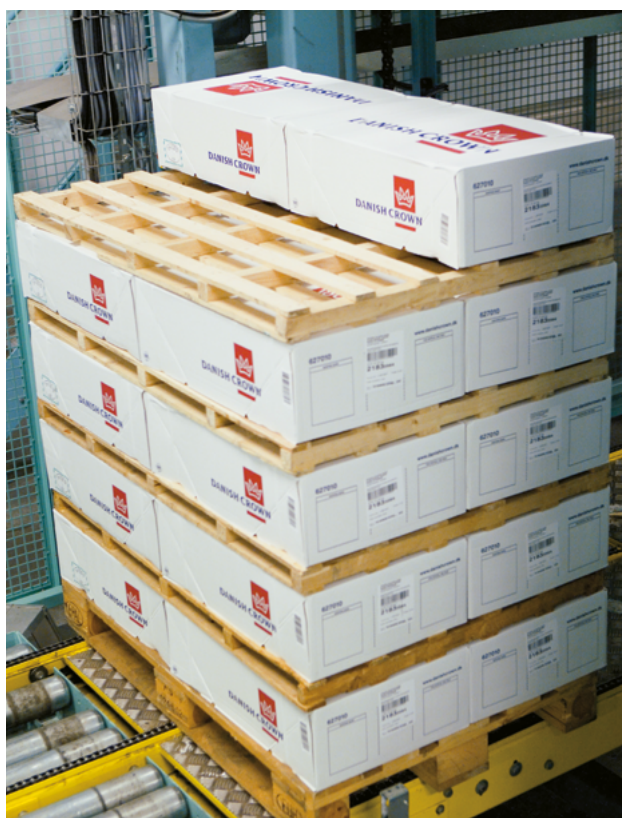
Cartons for freezing are stacked on pallets, at a short interval from one another, to enable rapid and effective freezing down of the meat.
