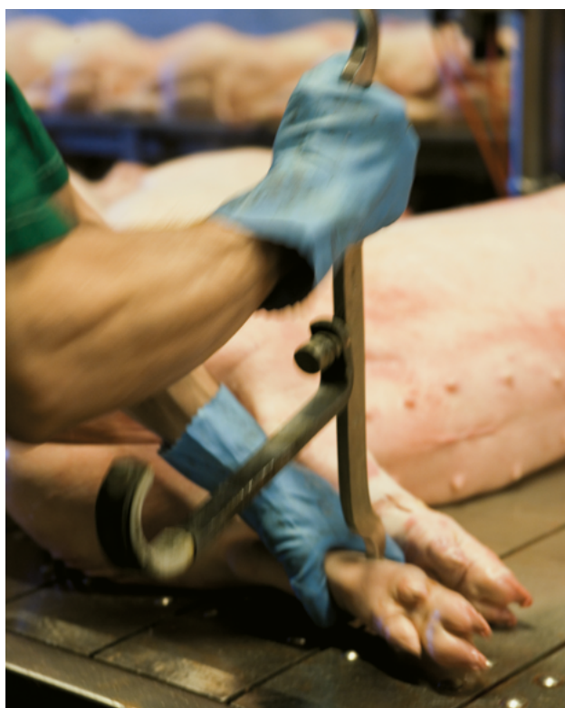
After dehairing, the carcass is hung on a numbered gambrel, which enables its automatic identification during the whole process until cutting.
