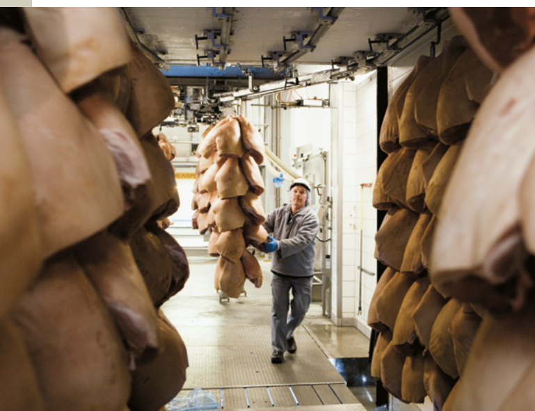
Cuts for further delivery are moved into cold storage or directly onto transport vehicles. The temperature must not exceed 7 °C.
