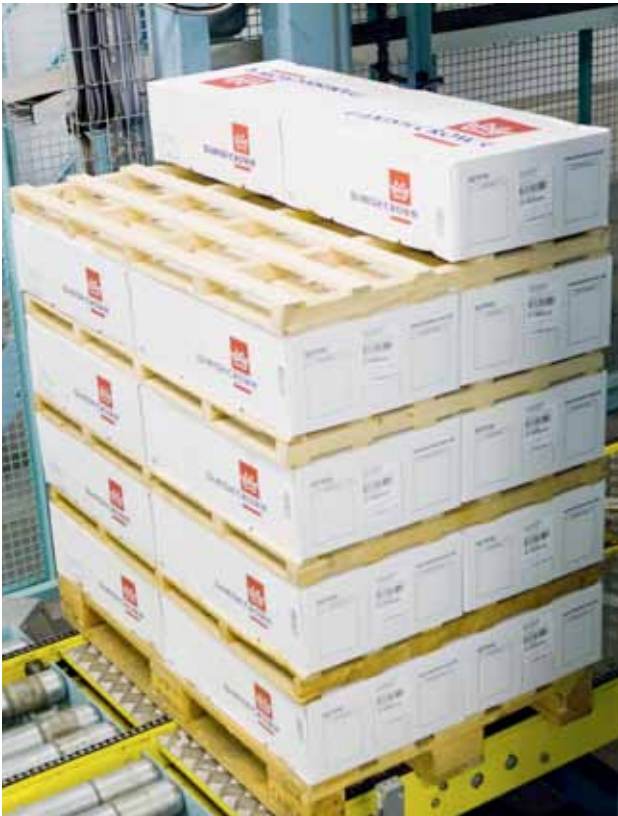
Cartons for freezing are stacked on pallets, at a short interval from one another, to enable rapid and effective freezing down of the meat.
