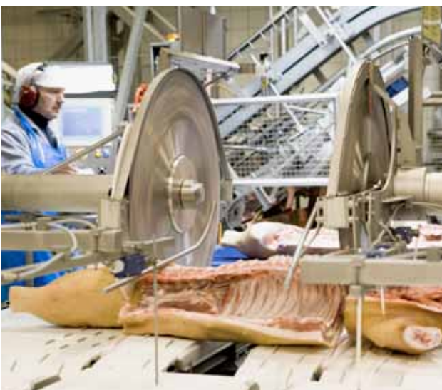
Each half carcass is then split in three parts. Laser light or phototechnology is used to ensure its correct positioning, before being divided into the three primal cuts: the fore-end, the middle and the leg.
