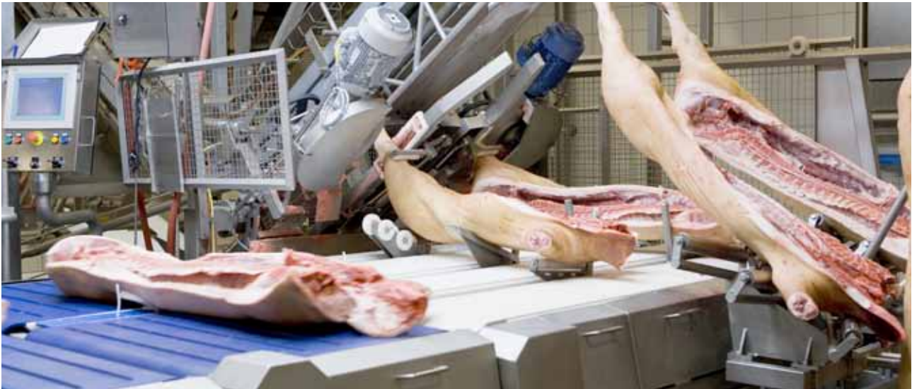
The two half carcasses are automatically lowered onto a conveyor belt, after which the hind toes are sawn off.
