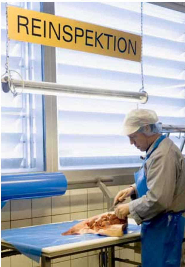
At the re-inspection procedure, any segregated or discarded cuts are examined and subsequently returned or sent on for alternative types of production. All trimmings must go for rendering. Only experienced personnel may carry out the task of re-inspection.
