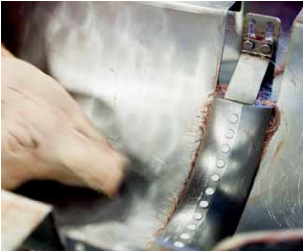
Autofom calculates the meat and fat content of the carcass, based on ultrasonic measurements. The measurements are performed by 16 transducers mounted on a channel over which the carcass passes once it has been transferred to the gambrel.
