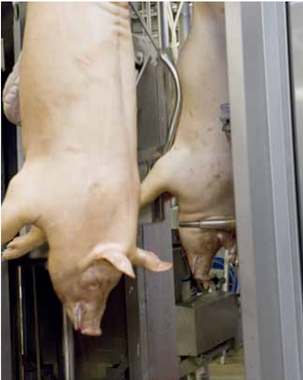
A process for the automatic removal of organs has been developed. The plucks and intestines are removed together by a machine and are then separated manually, away from the carcass itself. This procedure removes a burdensome task for the operator and is more hygienic than previous methods. The new equipment is not yet installed in all slaughterhouses.
