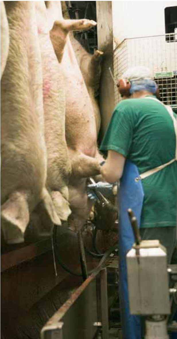
After stunning by CO 2 , sticking and bleeding take place by cutting the carotid arteries without the animal regaining consciousness.
