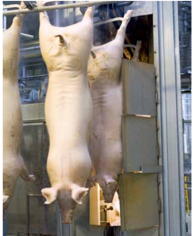
Typically, singeing of the carcass takes place in a furnace at 1000 °C for 6 seconds, thus eliminating bacteria, the remains of bristles and other dirt and preparing the surface of the rind for scraping.
