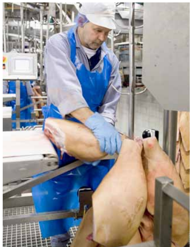
Cuts for further delivery are hung on a 'Christmas tree'. The hanging rails can be adjusted vertically to ensure that the cuts are hung properly.
