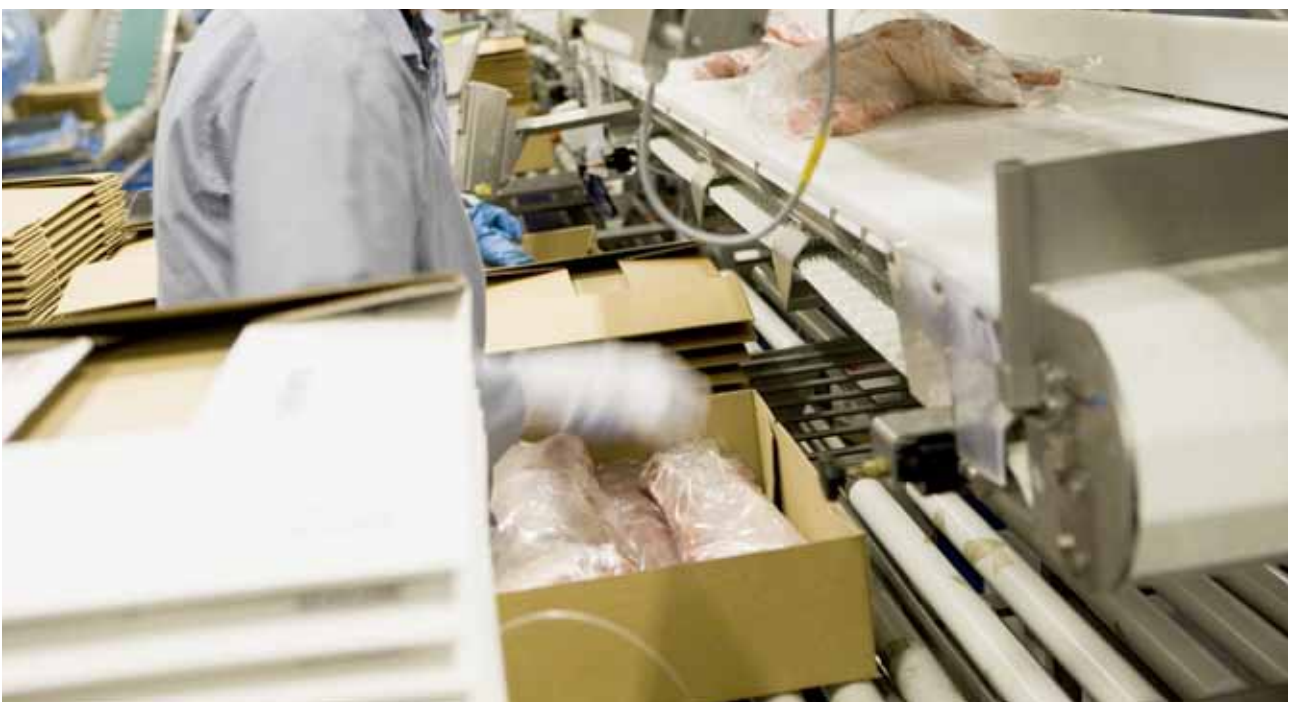
Finished cuts are immediately wrapped with film after which they are placed in cardboard packing, either by weight or number depending on customer requirement.
