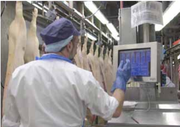
Observations by the veterinary inspectors are recorded electronically by linking to the gambrel number.
